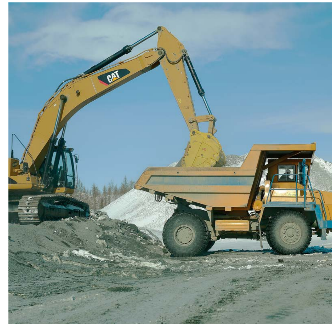
SUPER REINFORCED ROCK-DUTY BUCKET EXTRA 2,25 CUBIC METERS/CAT 349DL
