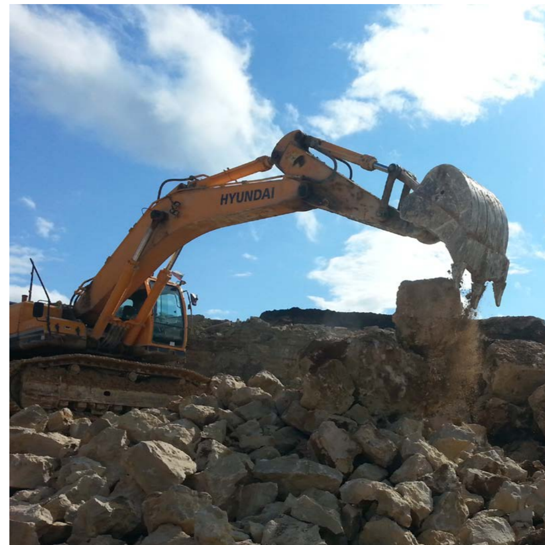
RIPPING BUCKET 1.04 CUBIC METERS/HYUNDAI R305LC-7
