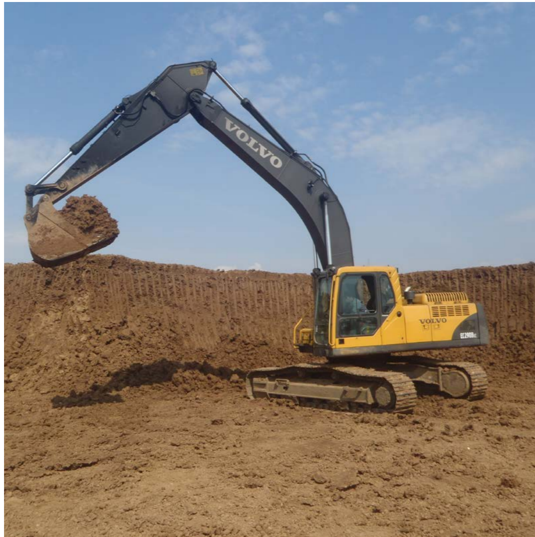
STANDARD BUCKET 1,25 CUBIC METERS/VOLVO EC-290
