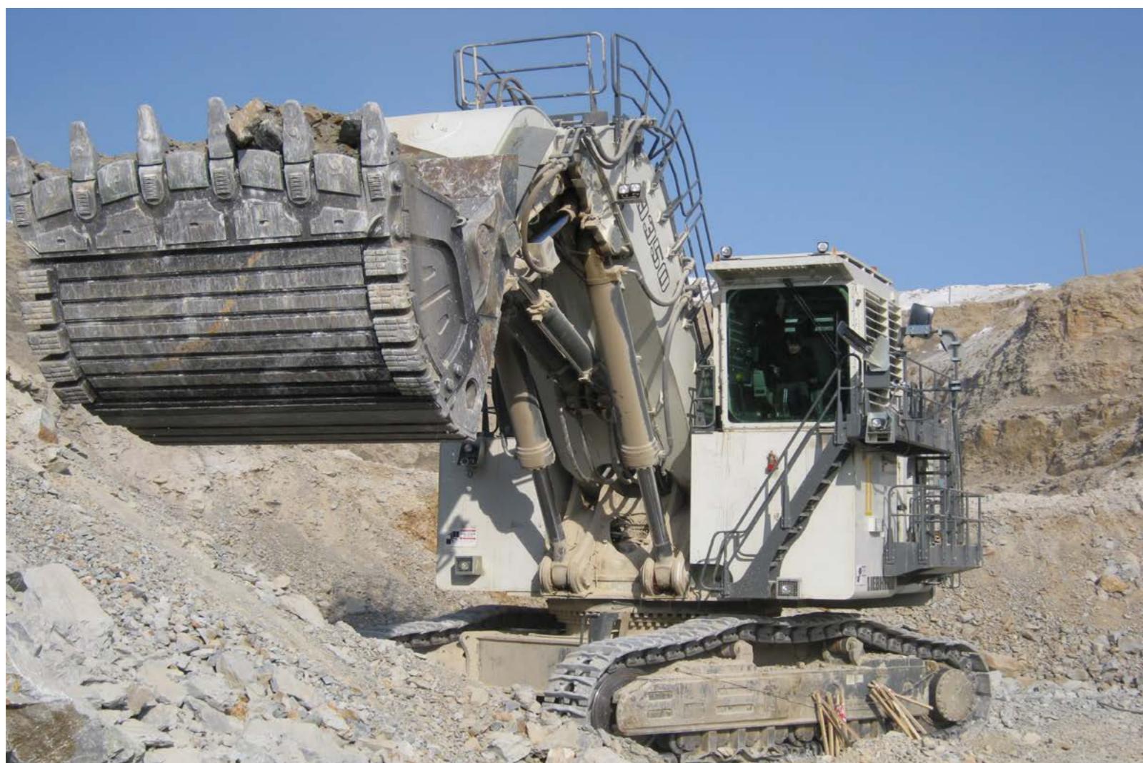
“FRONT SHOVEL” BUCKET 17,0 CUBIC METERS/LIEBHERR R9350
