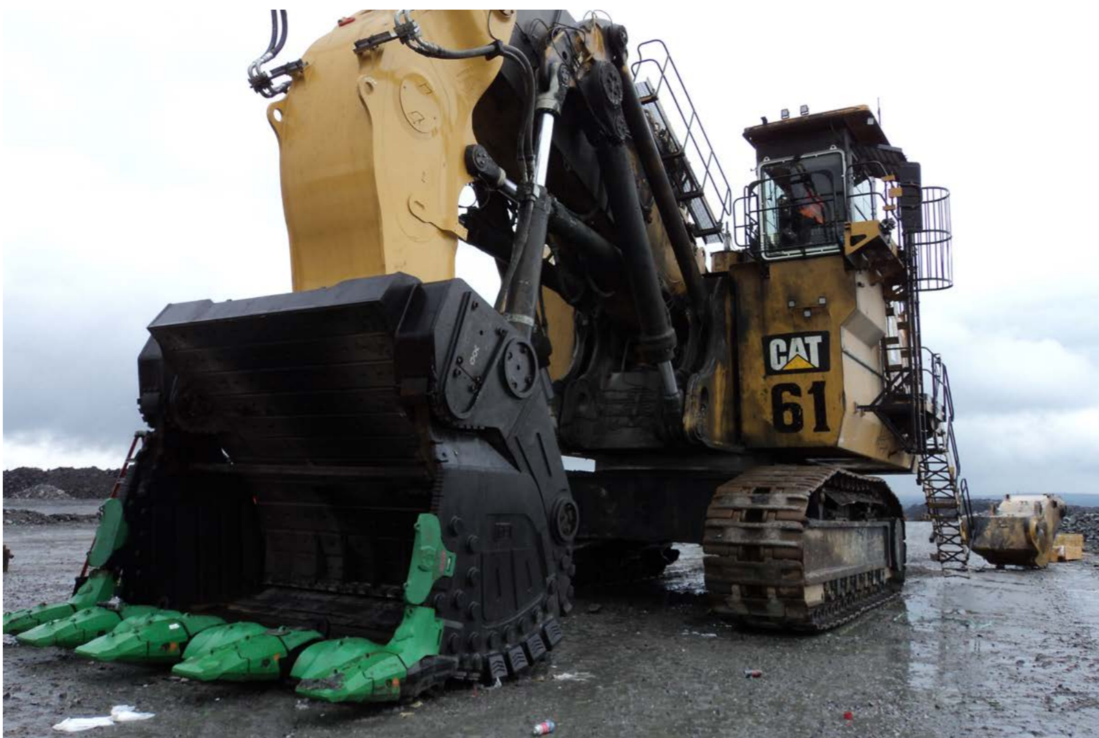
“FRONT SHOVEL” BUCKET 28,0 CUBIC METERS/CAT 6060
