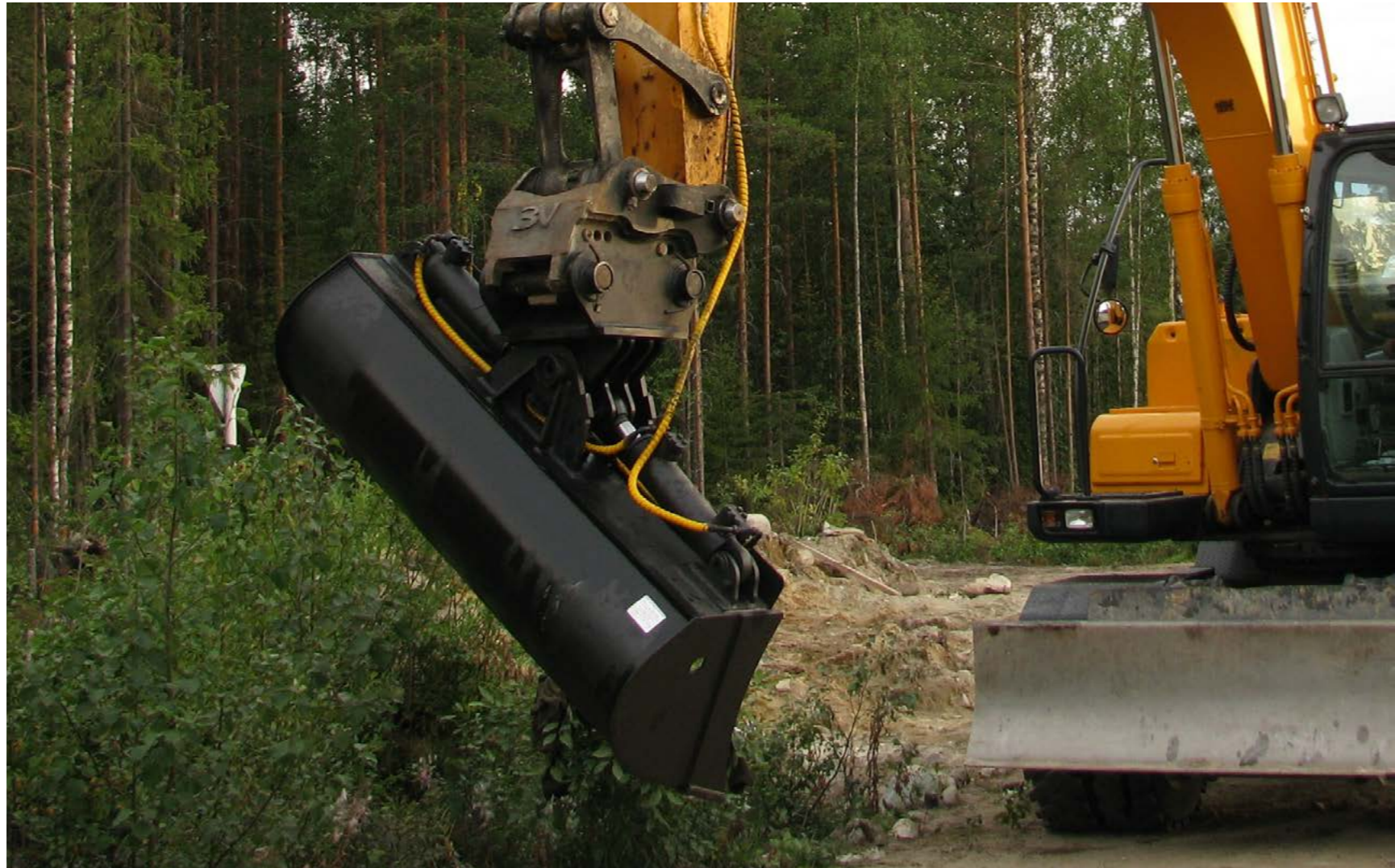
GRADING BUCKET WITH HYDRAULIC ROTATION HYUNDAI R-170W
