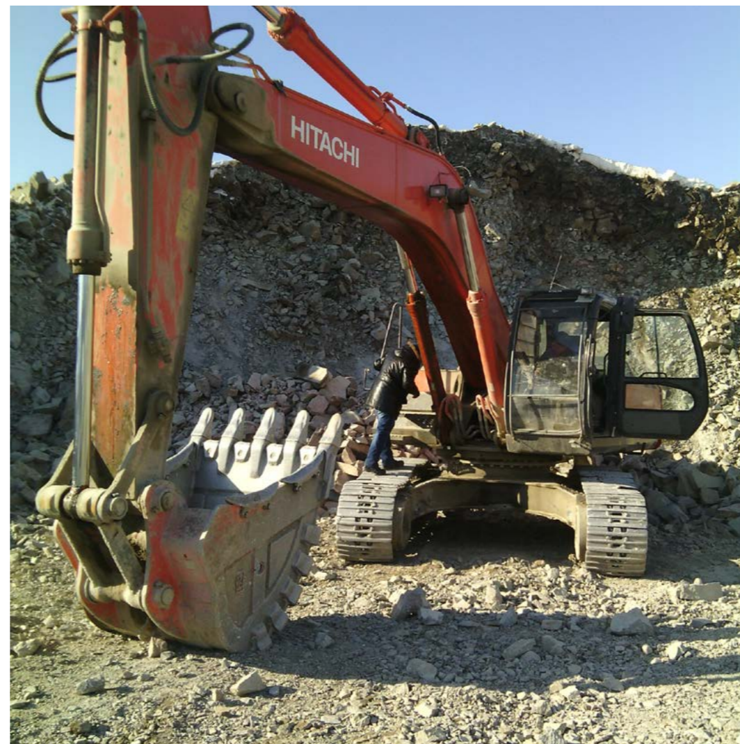
SUPER REINFORCED ROCK-DUTY BUCKET 1,4 CUBIC METERS/HITACHI ZX-330
