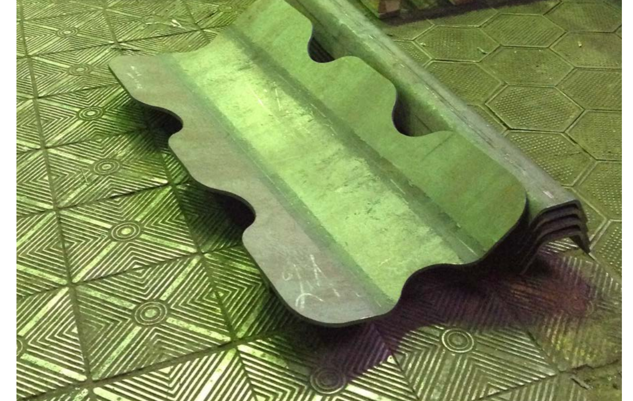
METAL BENDING PRODUCTION OF IRREGULAR SIZE BEAM CHANNELS
