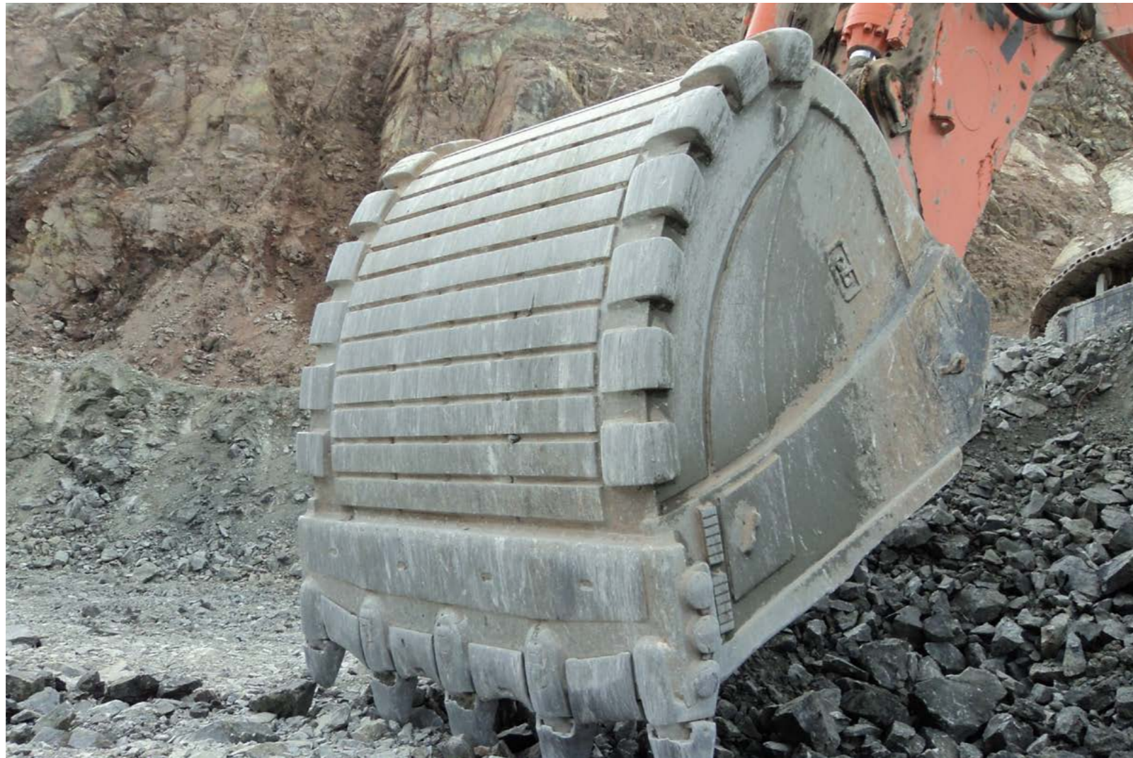
“BACK HOE” BUCKET 15,0 CUBIC METERS/HITACHI EX2600
