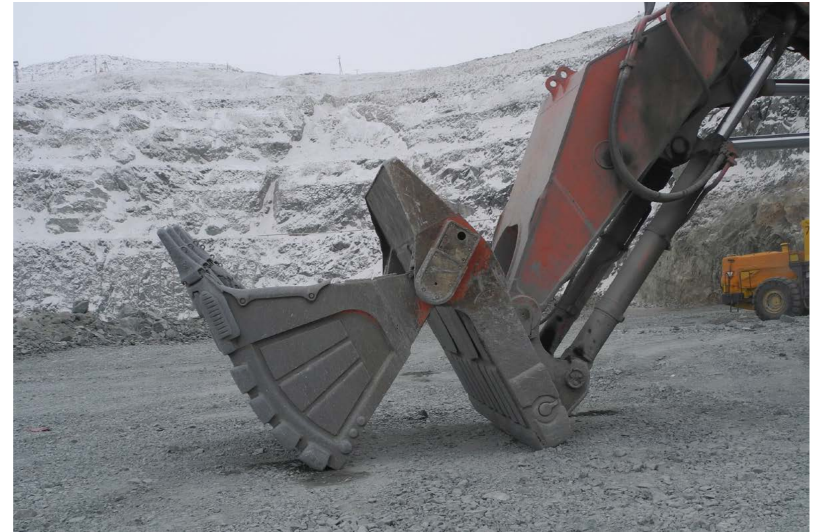
“FRONT SHOVEL” BUCKET 11,0 CUBIC METERS/HITACHI EX1900
