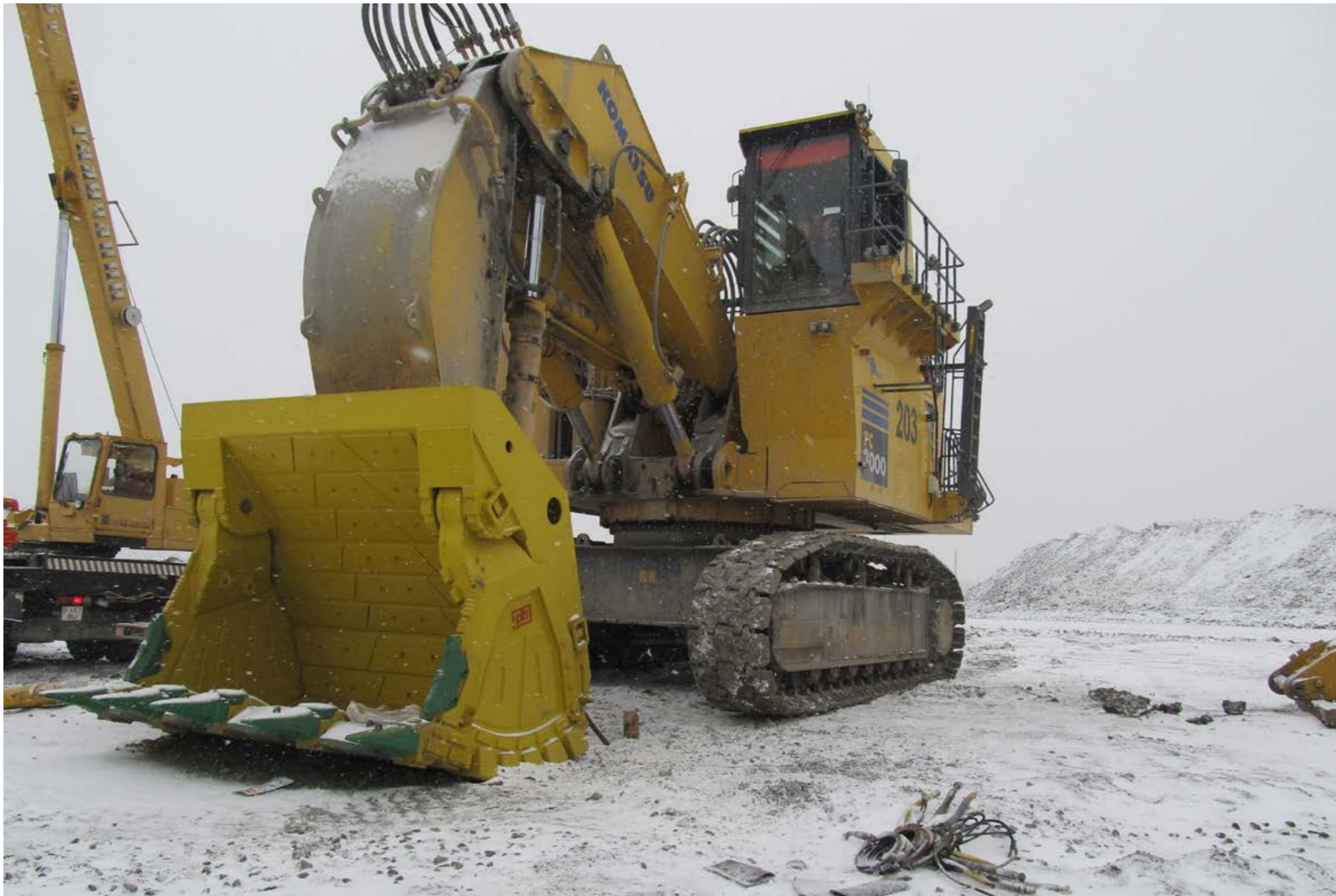
“FRONT SHOVEL” BUCKET 15,0 CUBIC METERS / KOMATSU PC3000
