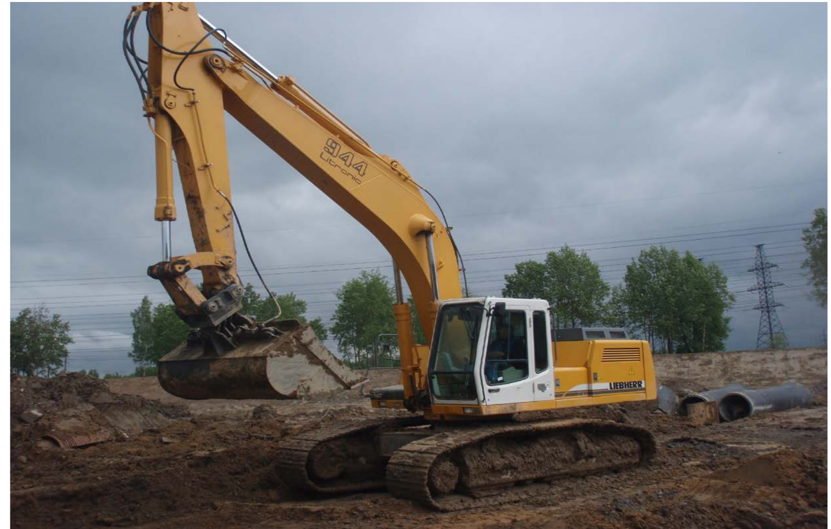
GRADING BUCKET WITH HYDRAULIC ROTATION LIEBHERR 944
