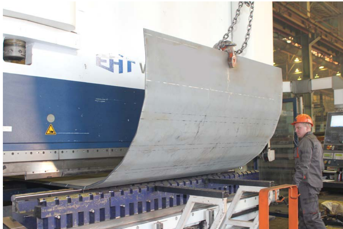
SHEET BENDING PRESS “EHT” (GERMANY), TRUMPF VARIOPRESS 800
