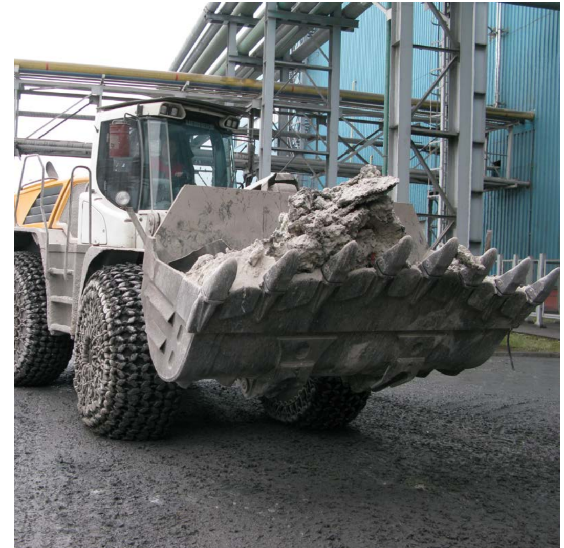
FRONT SUPER REINFORCED BUCKET 2,5 CUBIC METERS/LIEBHERR L556
