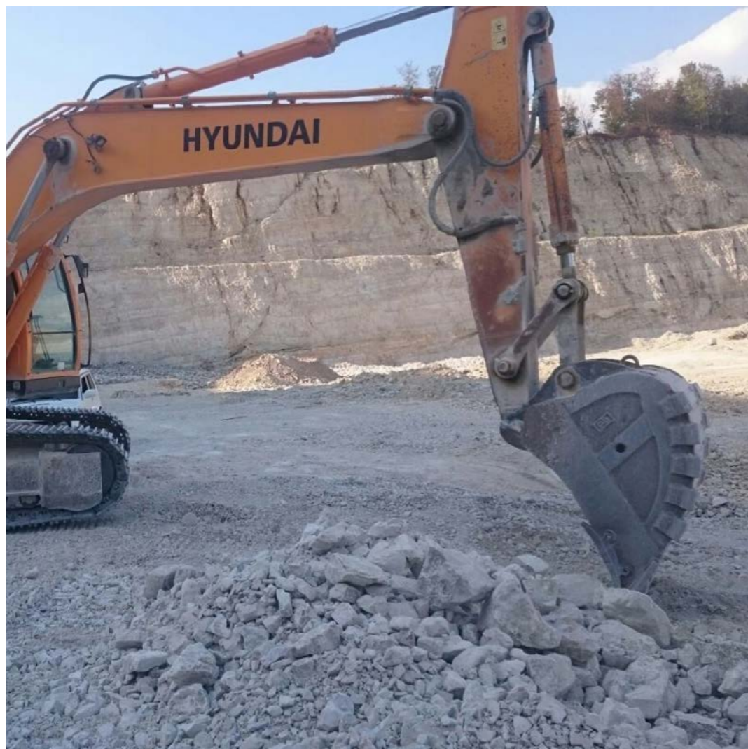
REINFORCED ROCK-DUTY BUCKET 1,5 CUBIC METERS/HYUNDAI R330-9
