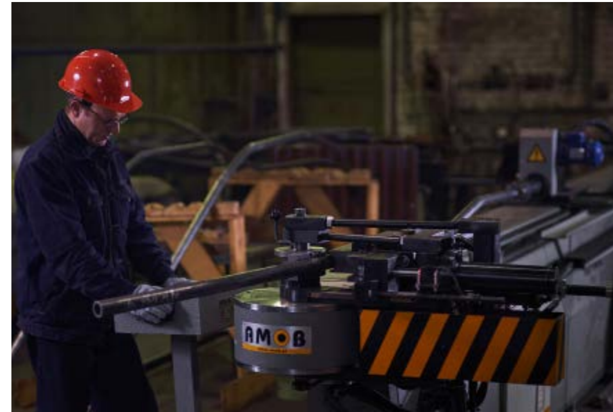
PIPE-BENDING MACHINE FOR PRODUCTION OF HYDRAULIC CIRCUIT
