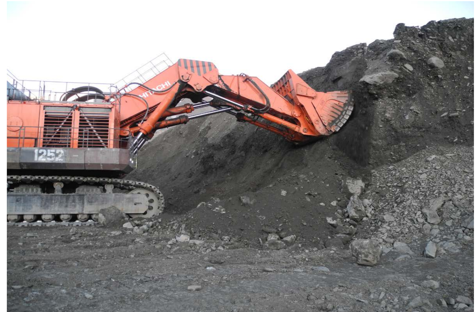
“FRONT SHOVEL” BUCKET 23,0 CUBIC METERS/HITACHI EX3600
