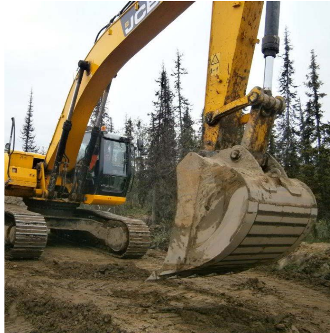
REINFORCED BUCKET 1,65 CUBIC METERS/JCB-330
