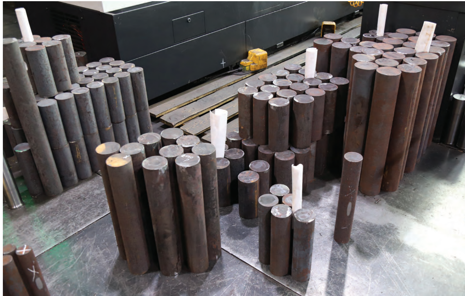
Blank parts for further axles, pins and bushings` production
