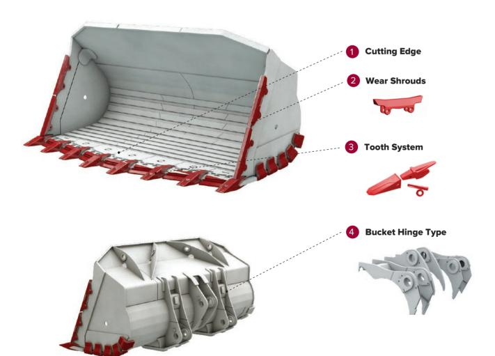
Wheel loader FLR Series and FLRX Series Rock Buckets equipped with reinforced protection package are built by Professional LLC for all brand machines. Exact type of protection elements that increase bucket durability significantly will be offered to a Customer depending on requested digging force, soil density and other factors.
