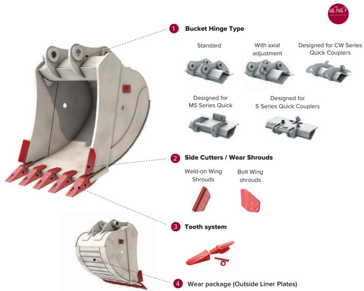
**GP Series Standard Buckets** are designed for construction pit and quarry operations (I - IV Soil Classes) and are used in bulk earthworks including excavation of materials (density up to 1600 kg/m³) such as: sand, loam, organic matter and crashed stone.
